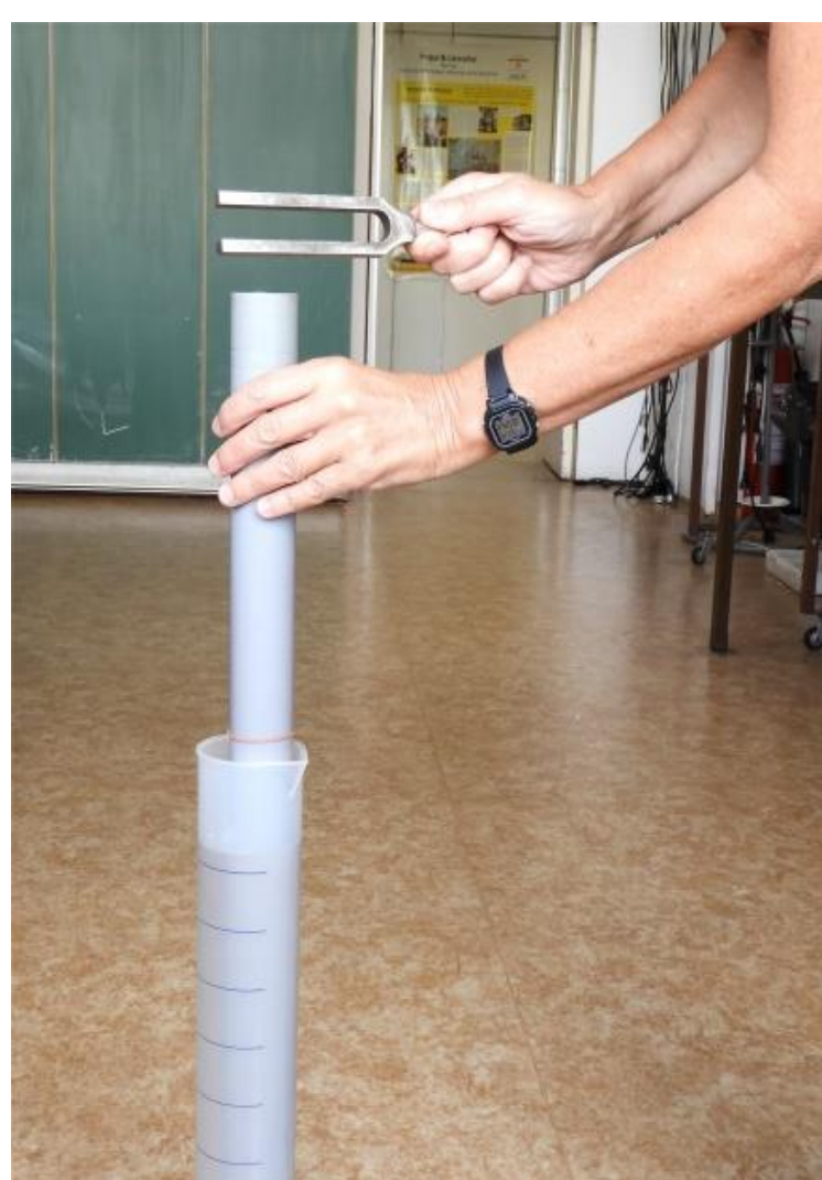
Measuring the speed of sound in the air: v = \lambda f = 2df
